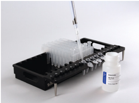
Figure 2. Setup and configuration of the deck tray(s). Elution Buffer is added to the elution tubes as shown. Plungers are in well #8 of the cartridge.
