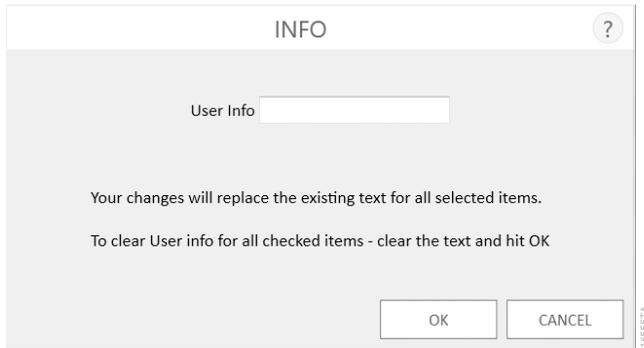
**Figure 14. 'Info' screen.** After selecting a protocol(s) and pressing the **Info...** button, the 'Info' screen is displayed. Touch the User Info text box to show an on-screen keyboard. Enter any identifying text to associate with the selected protocol(s), then press **OK** or **Enter** on the keyboard. Press the **OK** button on the 'Info' screen to associate this text with the selected protocol(s) or press the **Cancel** button to discard any changes.
