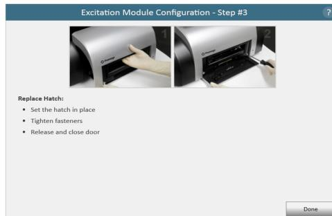
**Figure 94. Replacing the hatch door.**
