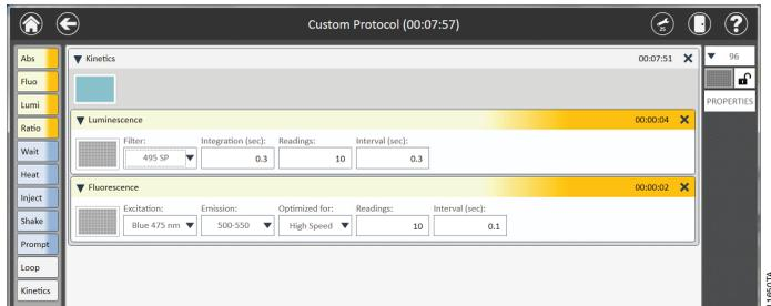
**Figure 36. Steps contained within a kinetic function.**
