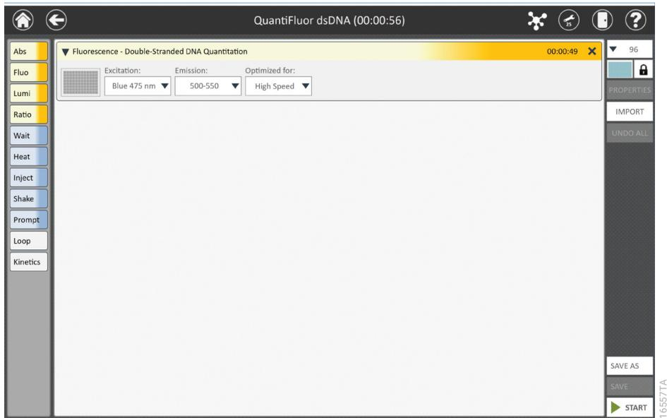
**Figure 41. Protocol-specific screen.** After selecting a preset or user-defined protocol, the individual steps of the protocol are displayed on a protocol-specific screen. Press the **Import** button on the right side of the screen to import a plate map.
