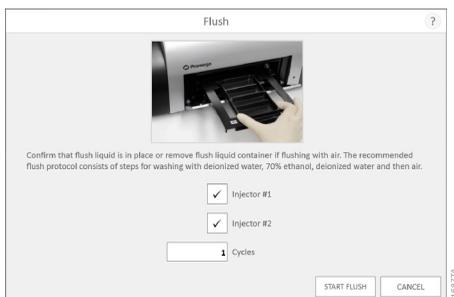
**Figure 123. Injector Flush function.**
