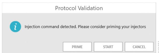
**Figure 53. 'Protocol Validation' screen.** When a protocol contains injector steps, the 'Protocol Validation' screen is displayed to allow the user to prime the injectors before starting the protocol.
