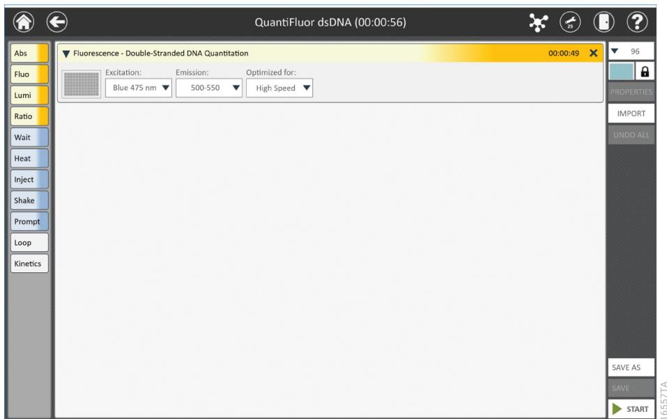
**Figure 46. Protocol-specific screen.** After selecting a preset or user-defined protocol, the individual steps of the protocol are displayed on a protocol-specific screen. Press the **Import** button on the right side of the screen to import a plate map.
