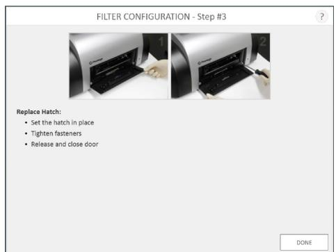
**Figure 91. Replacing the hatch door.**
