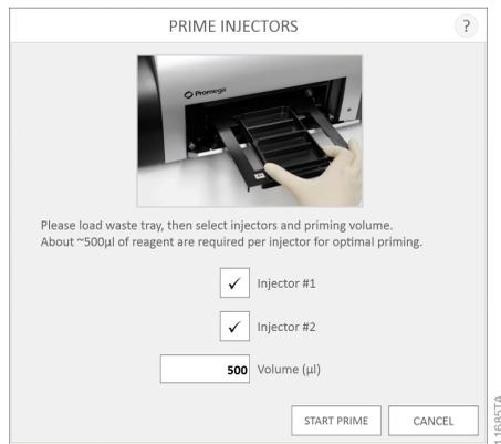
**Figure 121. Injector prime function.**
