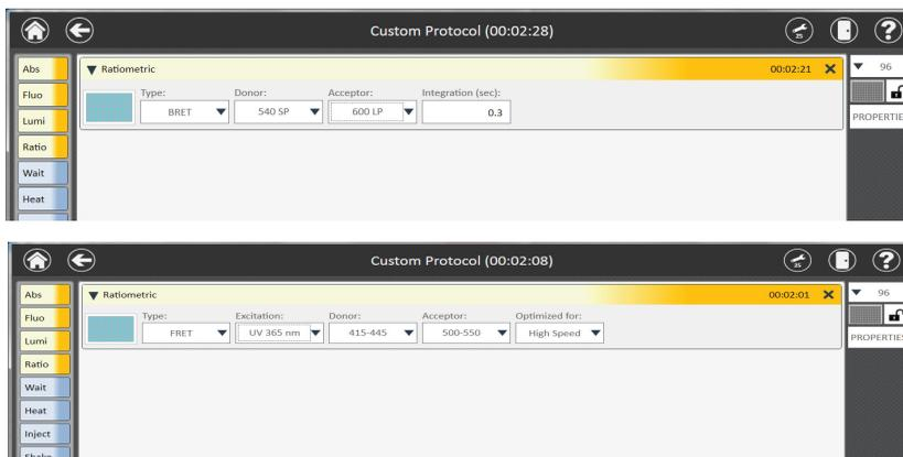
**Figure 25. Ratio function for BRET and FRET reads.**
