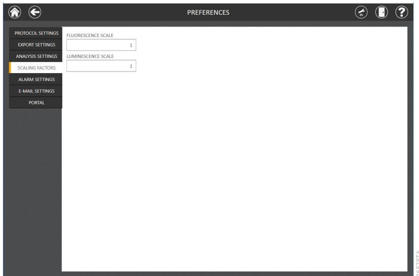
**Figure 104. Scaling Factors tab.** Administrators can specify a multiplier of 0.001 to 1000 that should be applied to fluorescence or luminescence data produced by the GloMax<sup>®</sup> Instrument.
