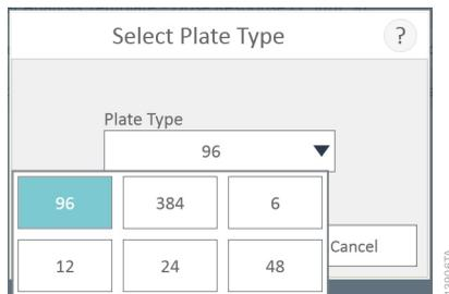
**Figure 65. The 'Select Plate Type' screen.** When creating a new analysis template, the first step is to select the plate format for the analysis template from the drop-down list on the 'Select Plate Type' screen.
