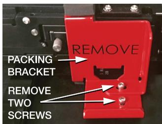
5. After removing the red Packing Bracket, remove the blue Packing Bracket Mount, and ensure the instrument is free of any packaging material parts.
